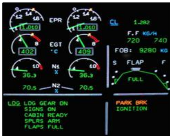
Figura 2: ECAM (Eletronic Centralized Aircraft Monitor) do A320
