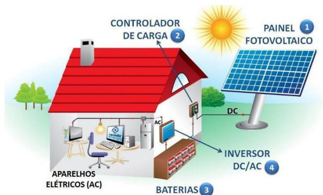
Fig. 5 - Sistema off grid [12]
