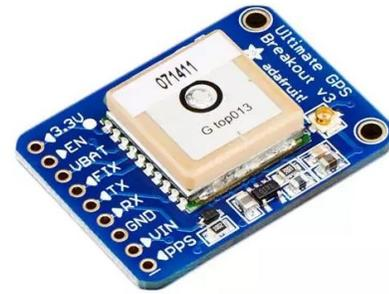
Figura 10 – Receptor GPS Breakout v3 adafruit.
