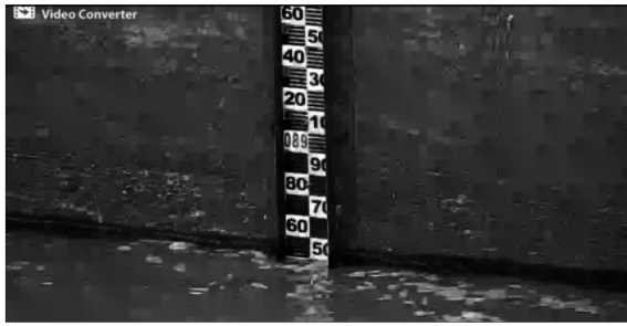
Figure 5: Contrast enhancement of the image from Figure 4 by Gamma Correction .
